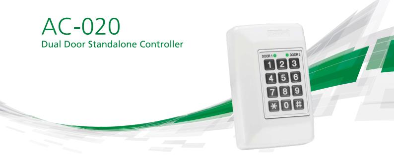
THE AC-020 CONTROLLER IS A COMPACT YET FULLY FEATURED SOLUTION FOR TWO-DOOR ACCESS CONTROL. IT SUPPORTS TWO READERS (IN/IN), TWO LOCK-STRIKES AND TWO REQUEST-TO-EXIT (REX) INPUTS. THE INTEGRATED POWER SUPPLY UNIT POWERS THE LOCKS AND READERS AND HAS A BUILT-IN BACKUP BATTERY CHARGER. THIS COMPACT AND COST EFFECTIVE UNIT IS EASY AND QUICK TO INSTALL. PROGRAMMING IS SET ON THE LOCAL KEYPAD. THE AC-020 IS COMPATIBLE WITH A WIDE RANGE OF READERS AND LOCK TYPES.
