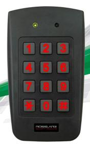
ROSSLARE'S NEWEST STANDALONE BACKLIT PIN & PROXIMITY CONTROLLER, THE AC-F44, IS A COST EFFECTIVE SOLUTION FOR INDOOR AND OUTDOOR SYSTEMS WHERE PIN AND/OR PROXIMITY CREDENTIALS ARE REQUIRED. THIS DURABLE MODEL CAN BE EASILY PROGRAMMED WITH UP TO 500 USERS ON A SINGLE DOOR.
