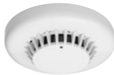
SA-61 Wireless Photoelectric Smoke Detector • Local alarm sounder • LED indicator for transmissions • Detector removal tampering and low battery messages
