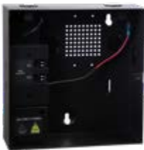
ME-0515M Multipurpose Power Management Enclosure • Two isolated output channels: 12 VDC at 2 Amp (4 Amps total) • Power Management Board with 7AH Lead Acid battery charger • Universal Input Voltage 100 VAC to 240 VAC 50/60Hz auto select • Tough metal enclosure featuring Rosslare's PowerLock™ C13 socket
